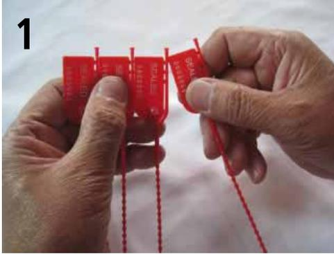
**1** Hold seal strip as shown. On seal being detached, place thumb only on seal-tab, NOT on tear-off rod. Now bend seal-tab and pull it apart from strip.
