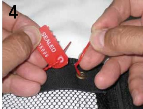
**4** Remove by pulling the tear-off rod away from the seal-tab and out of the grommets. The TR Kit cannot be re-sealed using the original seal.
